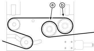
Fig 67 - Drive box, pinch roller (a) & drive roller (b)
