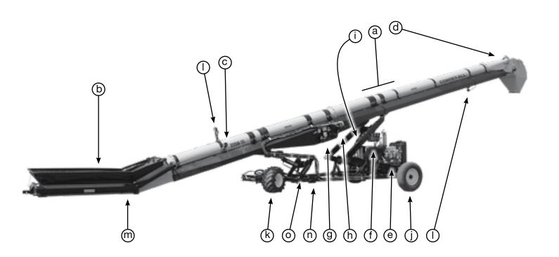
Fig 5 - 2250-TL Truck load conveyor
