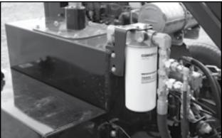
Fig 58 - Hydraulic oil filter
