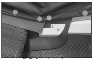
Fig 78 - Fasten flashing clamp
