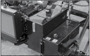
Fig 45 - Hydraulic oil reservoir and fuel tank
