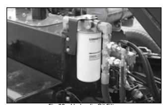
Fig 80 - Hydraulic Oil Filter
