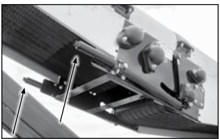
Fig 49 - Positive pinch drive tension bolts
