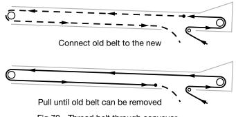
Fig 72 - Thread belt through conveyor
