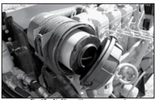
Fig 47 - Air filter with cover removed
