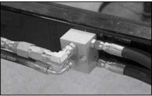
Fig 14 - Hydraulic manifold to drive wheel lift cylinder
