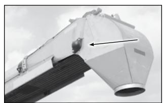
Fig 55 - Discharge roller bearings
