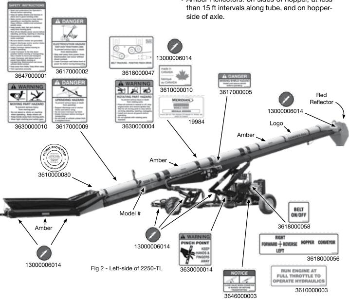
REMEMBER - If safety decals have been damaged, removed, become illegible, or parts were replaced without signage, new ones must be applied. New decals are available from your authorized dealer.
