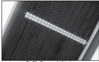
Fig 69 - Conveyor belt lacing
