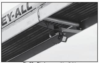
Fig 23 - Discharge working light
