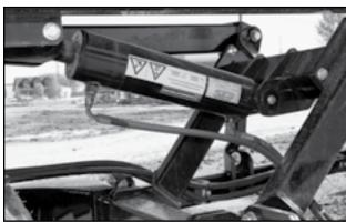
Fig 61 - Drive wheel lift cylinder
