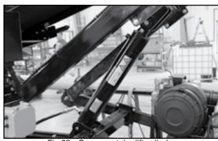
Fig 62 - Conveyor tube lift cylinder
