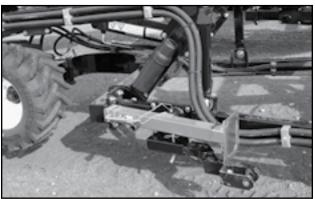
Fig 40 - Hitch and jack storage plate
