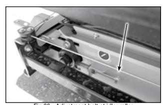
Fig 66 - Adjustment bolt at idler roller
