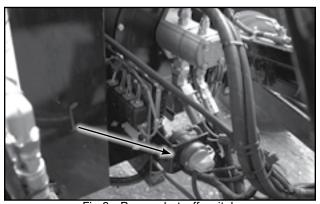
Fig 8 - Power shut-off switch
