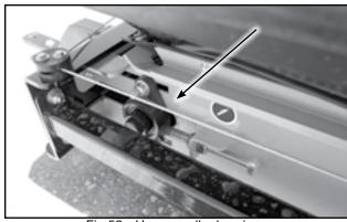
Fig 52 - Hopper roller bearings
