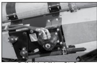
Fig 15 - Hydraulic Motor on Drive Box
