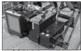
Fig 9 - Hydraulic oil reservoir and fuel tank
