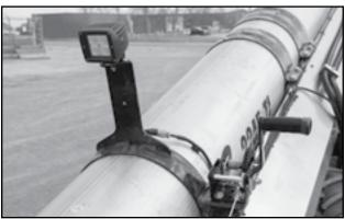
Fig 22 - Hopper working light
