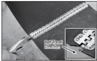
Fig 71 - Crimp lacing and taper belt corner
