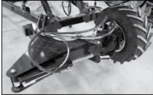
Fig 60 - Steering cylinder
