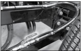
Fig 34 - Hydraulic ball valve to tube lift cylinder
